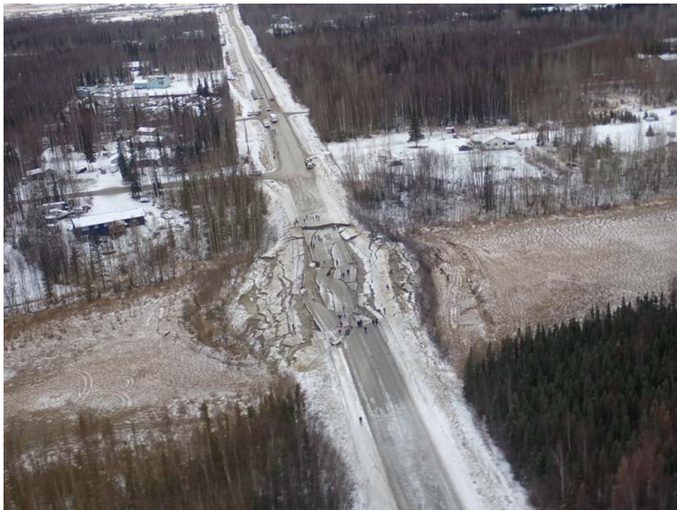
Photo 5. Lateral spreading disrupted Vine Road near Wasilla. Many failures of engineered materials occurred on or adjacent to saturated lowlands filled with organic sediment, silt, or sand. GPS position: 61.437615904°, -149.449646520° (Credit: Rob Witter, USGS)
