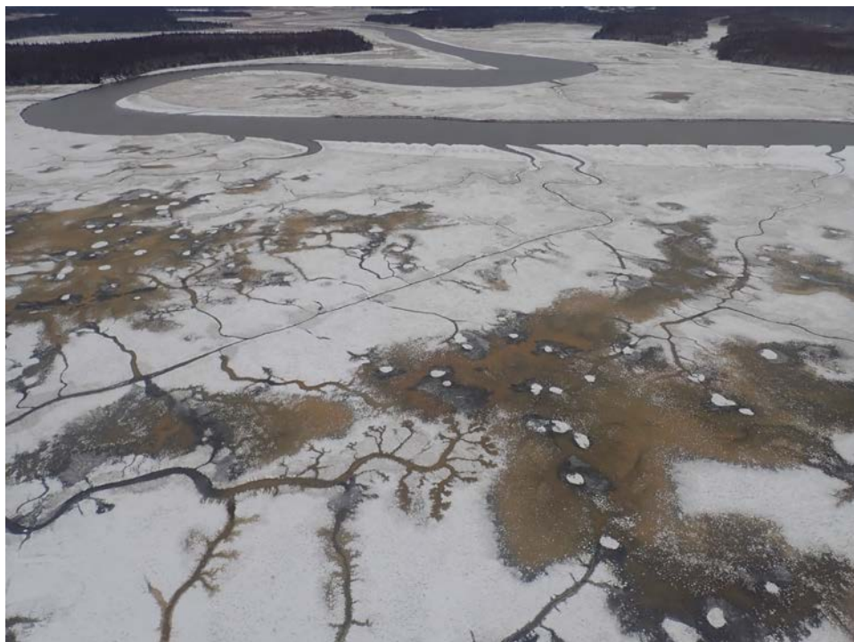
Photo 9. Sediment vented by earthquake-triggered liquefaction at the mouth of the Little Susitna River. GPS position: 61.420135331°, -149.220729268° (Credit: Adrian Bender, USGS)
