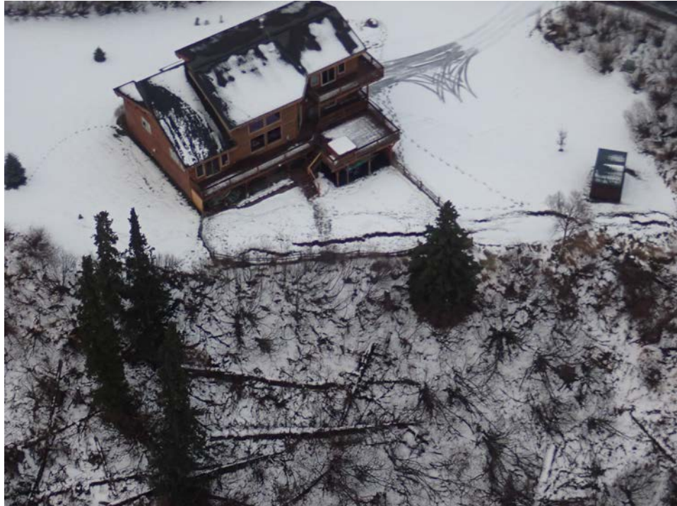
Photo 4. Ground cracks present the potential for future slope failure during aftershocks or heavy rainfall. These cracks occur at the top of a steep valley wall on the south side of Potter Creek in south Anchorage. GPS position: 61.437615872°, -149.449646563° (Credit: Rob Witter, USGS)
