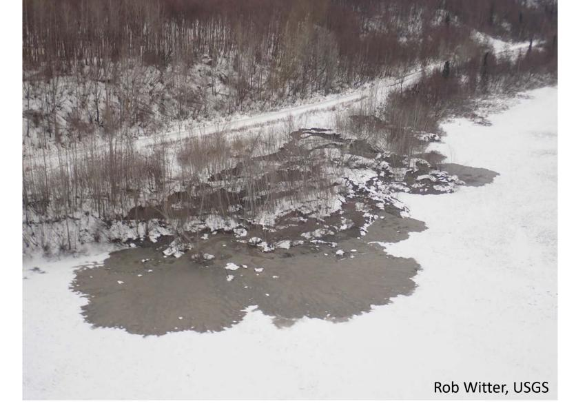
Complex earthflow slumping along Alaska Railroad overlooking tidal flats along Knik Arm near Mirror Lake. Failure of these low bluffs may have involved liquefaction.
