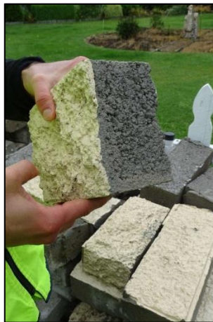
Heavy solid veneer cladding blocks
