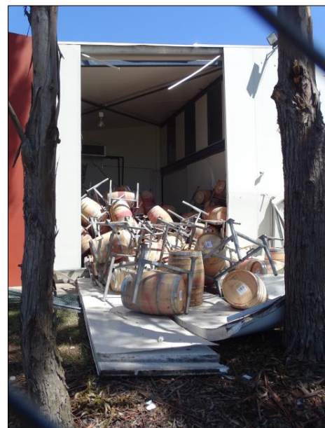
Collapse of stacking systems - wooded barrels' storage
