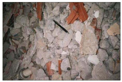
*Figure 19.* Substandard detached aggregate material in the debris of the collapsed Çeltiksuyu School building.
