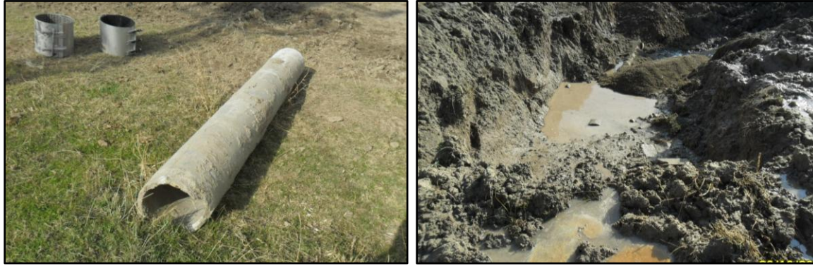
Figure 21. Pipe breaks and repaired sections in Topakca village due to liquefaction induced lateral spreading
