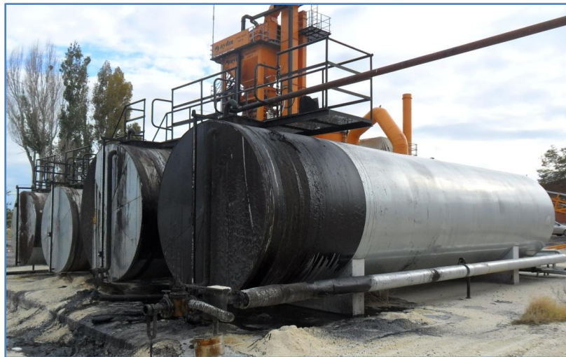
Figure 13. Overflow of asphalt in storage tanks (Ercis-Adil Cevaz highway)
