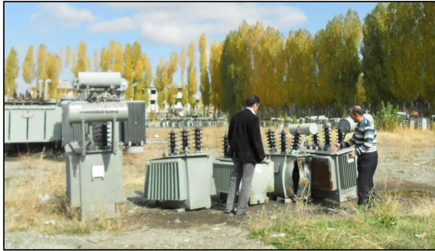
Figure 19. Burned/damaged 400 kW and 600 kW transformers due to fall from elevated locations
