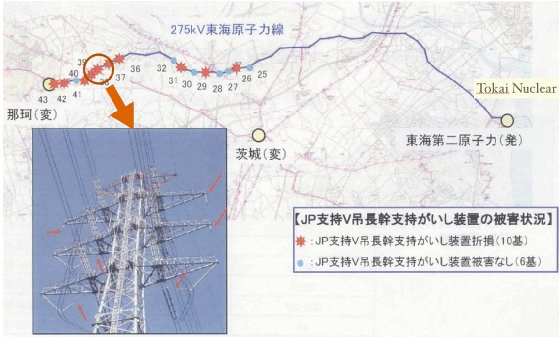
Figure 4-91. Damage to 275 kV Transmission Line
