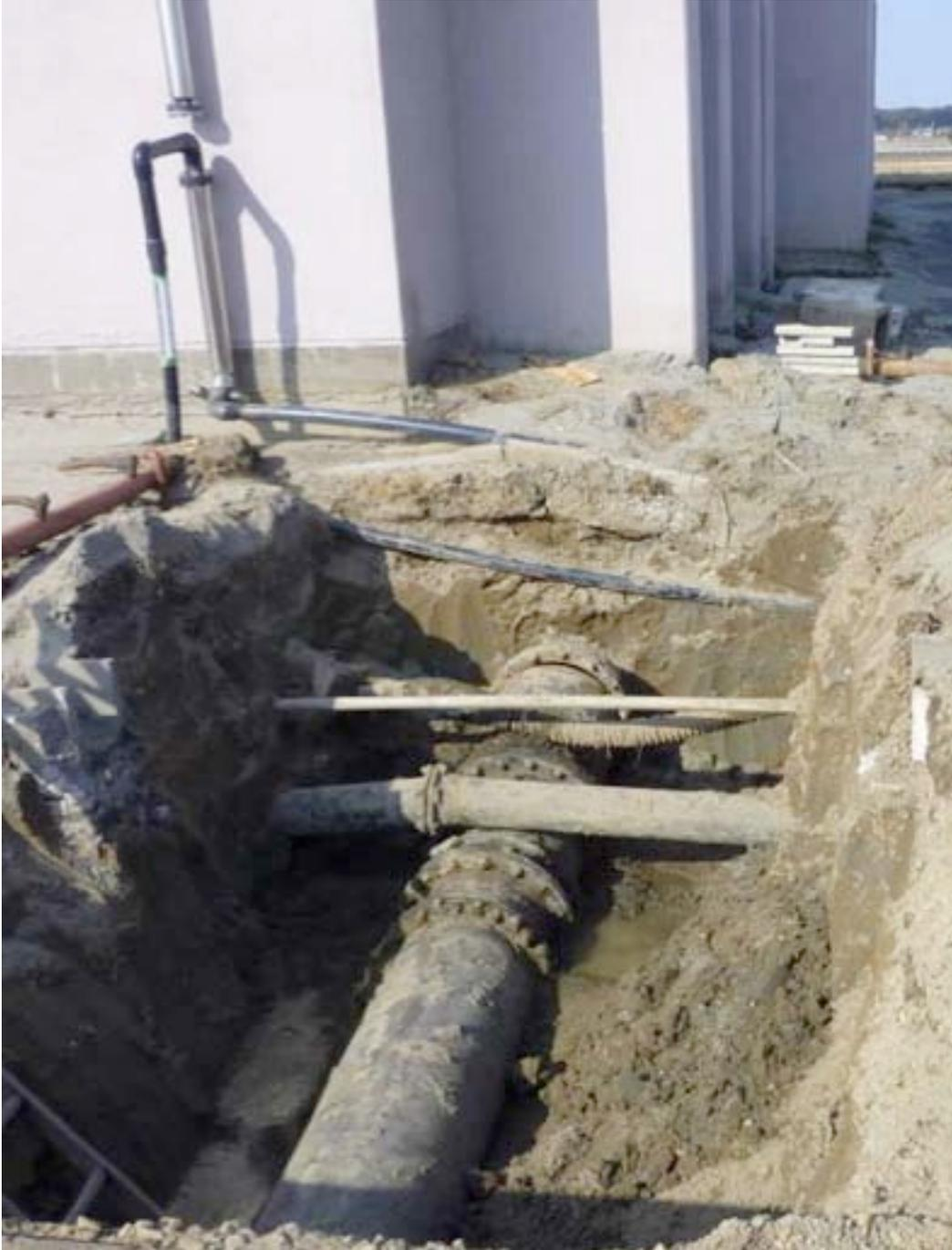
*Figure 3-38. Failed Pipe, Wanagawa WTP*
