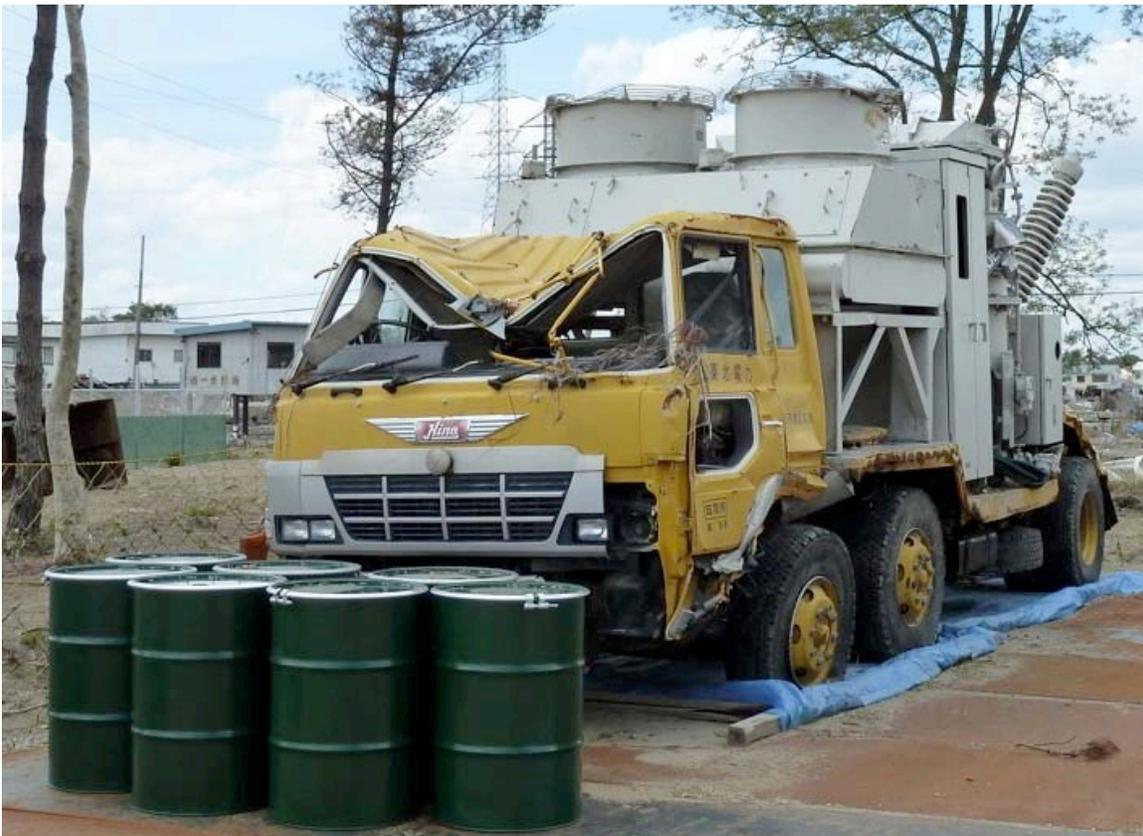
*Figure 4-59. Portable 66 kV Transformer Damaged by Inundation, Ishinomaki*
