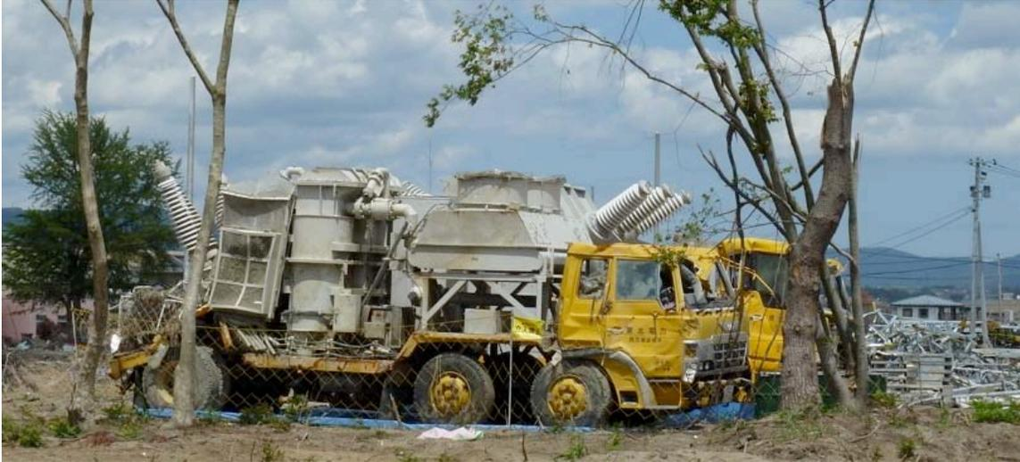
*Figure 4-58. Portable 66 kV Transformers Damaged by Inundation, Ishinomaki*
