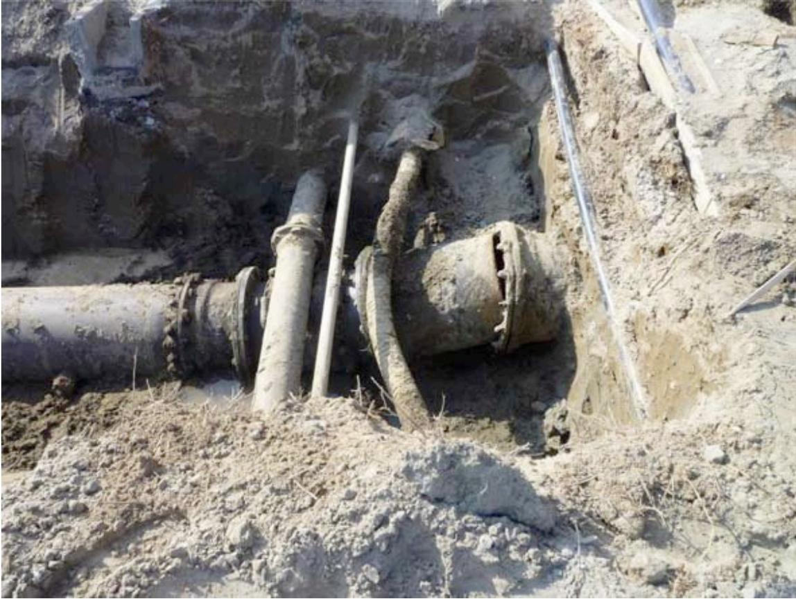
*Figure 3-37. Wanagawa Water Treatment Plant, Failed Pipe*
