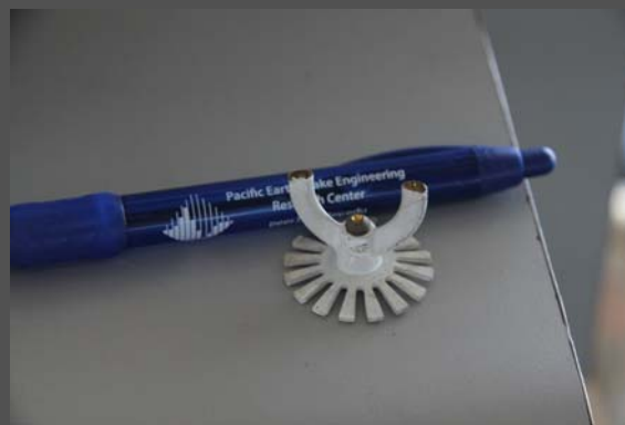
Closeup view of some sprinkler heads sheared off
