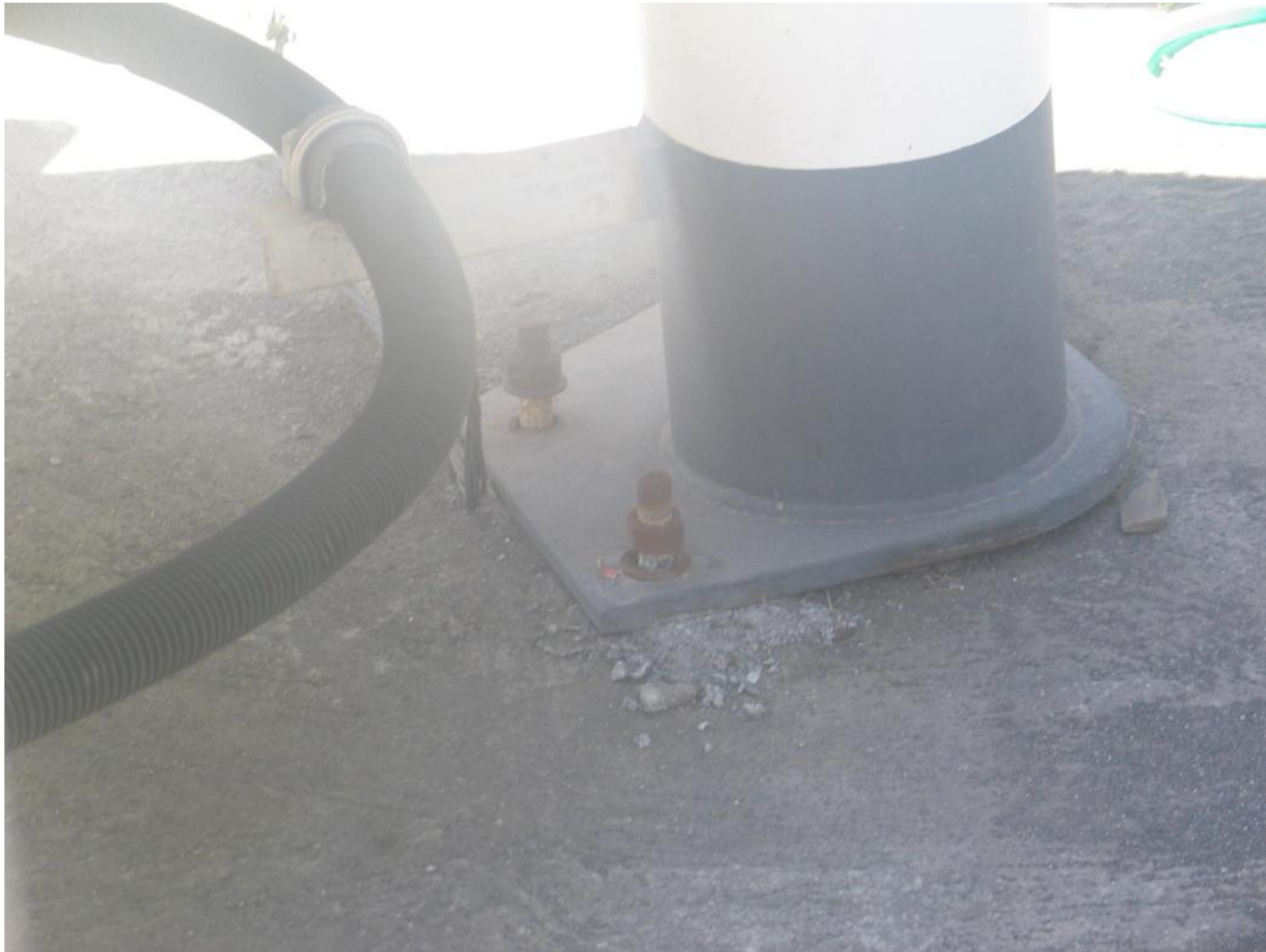
Overturning tension stretched anchor bolts. Talcahuano Hospital.
