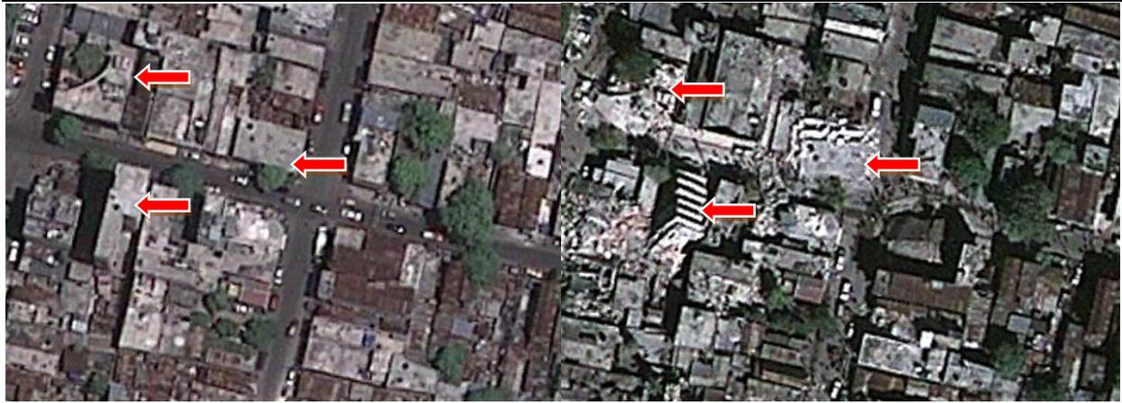
**Figure 6.5 Pre- (left) and Post-event (right) Imagery of “Pancaked” and “Stair-step” Damage Patterns**
