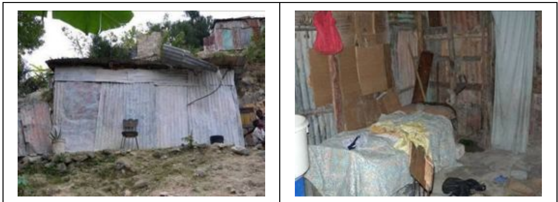
Figure 6 TCWR, Timber and corrugated galvanised iron walls and roof (similar to type T) also.
