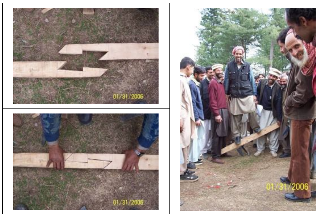
Figure 23 Good quality timber joinery and testing.
